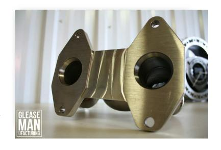
Our wastegate positions are crucial. This keeps from over-boosting at lower boost levels, and makes boost control smooth and predictable. The entries are tear dropped, which allows a larger, more directional flow into the wastegates.
