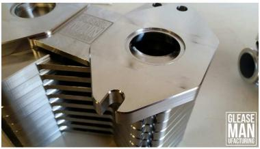
The last step of building these manifolds is sanding the flanges perfectly flat. This is time consuming to do properly on 304 stainless, but it's a critical step for a perfect seal and crack resistance. Torqueing an untrue manifold to an engine block will stress the primaries, and often results in cracking.
