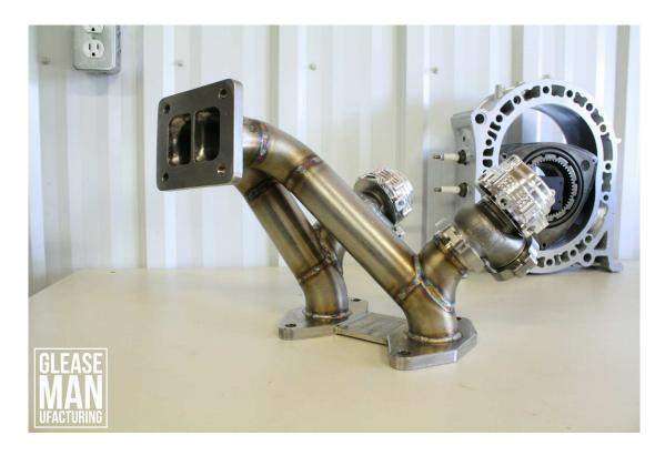
Our dump tubes are built to your wastegate selection and are a cheap and easy purchasable solution to exhaust the wastegates past the subframe.
