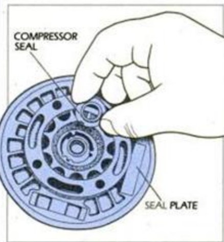
Rotate the positive multipart seal to release it from the seal plate.
