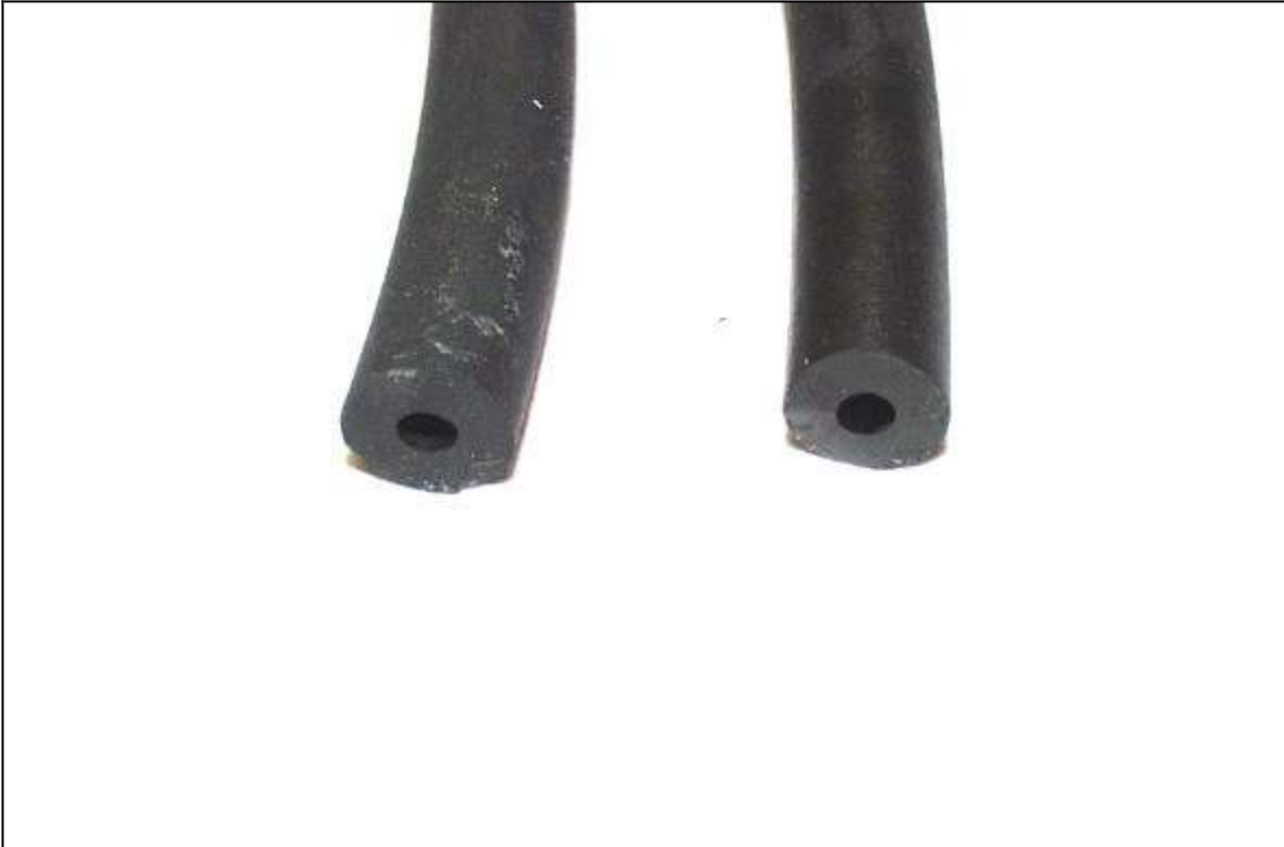
Figure 2. The Neoprene tubing on the left was not subjected to the hot oil. The tubing on the right was subjected to 240 °F for 1,000 hours. Although you can't tell from the picture, the tubing on the right has hardened to the point it can not be completely pinched off with your fingers. It is very stiff and non-rubber like.
