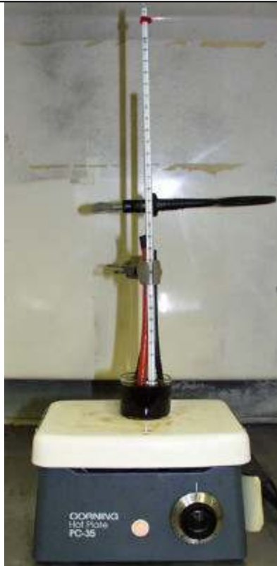
Figure 1. The test setup consisted of the three tubes suspended vertically. Approximately two inches of the tubing was immersed in the 30W-engine oil. The oil temperature was maintained at 240 °F for 1,000 hours.
