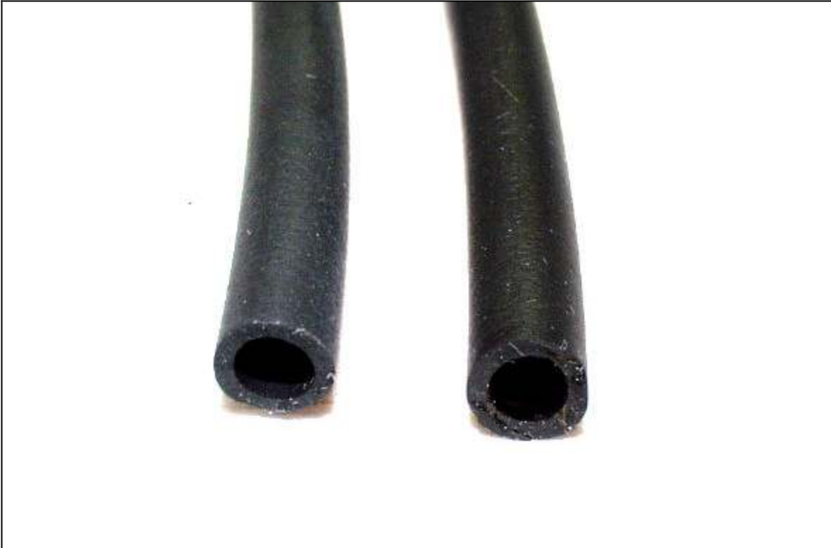
Figure 3. The Viton tubing on the left was not subjected to the hot oil. The tubing on the right was subjected to 240 °F for 1,000 hours. Other than a film of oil coating the surface there is no difference between the tubes. The elasticity, hardness and strength were not degraded.
