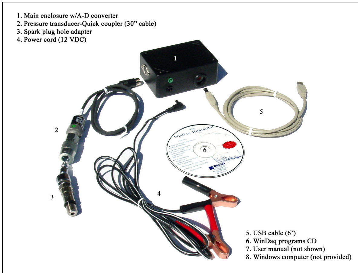
Figure 1. Rotary-engine Compression Tester system Model ReCT-03b components 1 .
