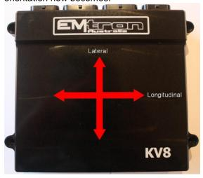
Longitudinal **positive** g-force = Acceleration. Typical values 0.3 to 0.5g Longitudinal **negative** g-force = Braking. Typical values: -1.5 to -1.8g
