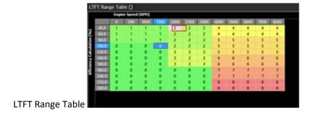
It is improtant to know these trim values are only loaded whilst the ECU is powered up. The LTFT values always reset once the ECU powers down. Future revisions will offer the option for the ECU to store the LTFT values permanently. Ideally the tune should be calibrated so to yield as close to 0% in all the LTFT tables.
