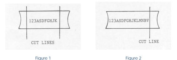
Unless otherwise specified, trim Protection Sleeve so that it is 10mm longer than the Marker Sleeve.
