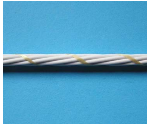
NOT ACCEPTABLE Lay length of Binder too long
