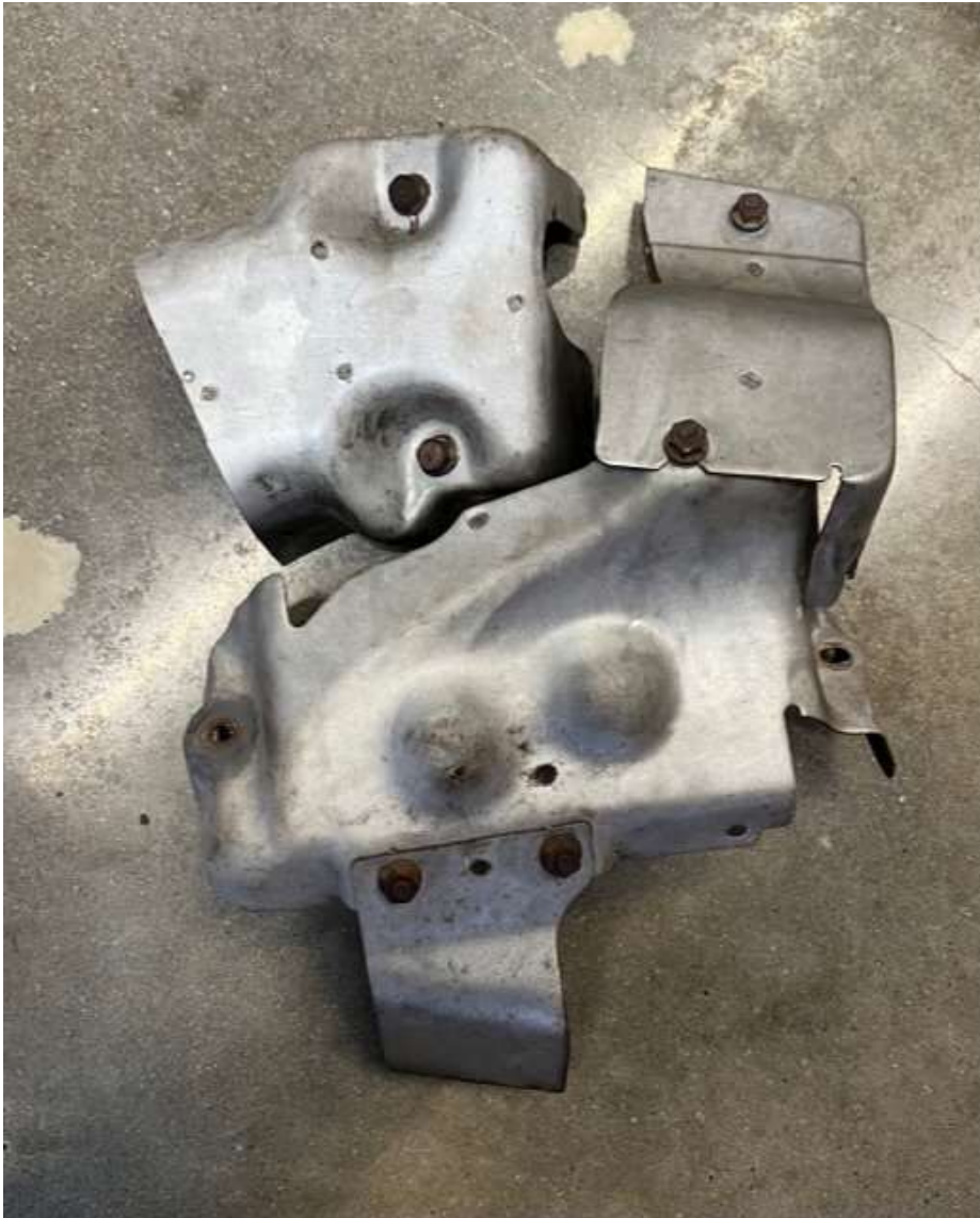
Pre-cat shield is in the upper left of the photo above.
