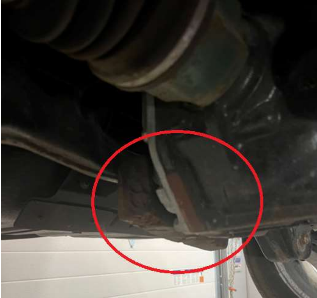
Block of wood behind rear of differential.
