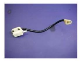
The clutch safety switch is no longer available, but the Miata safety switch part number FB01664D0 shown above will fit with some modification. The wires come out the wrong side and interfere on the LHD cars, so one must clip the plastic post the wires are tie strapped to and fold them down and glue them with epoxy.
