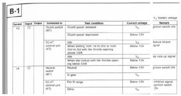
Clutch Pedal switch (B1-52), Page Z-35
