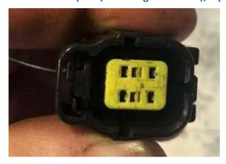
This sensor has 4 wires on it, 2 blue (1 $^{\rm st}$  gear)and 2 green (2 $^{\rm nd}$  gear)
