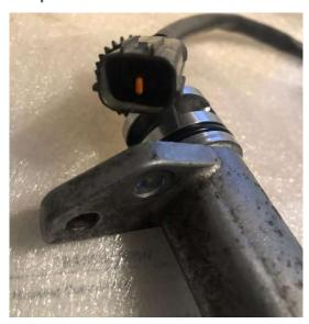
The Manual Transmission speed sensor drives the speedometer and it can plug directly into the AT vehicle harness.
