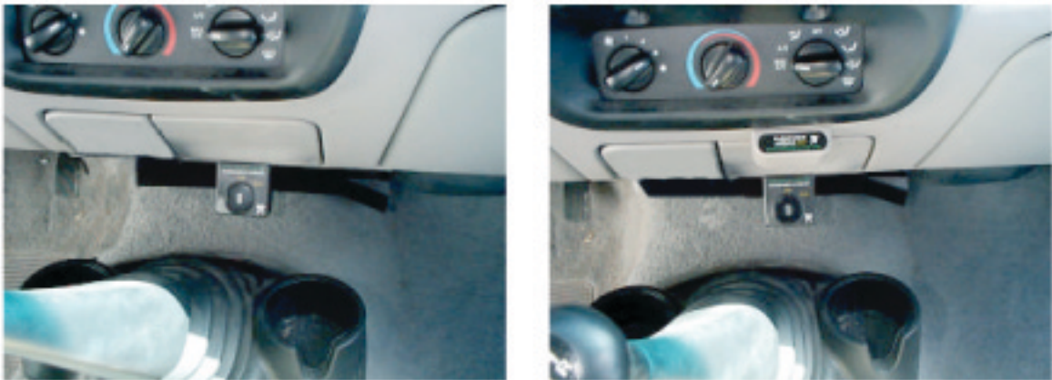
FIGURE 4 – UNDER THE DASH SWITCH MOUNTING
