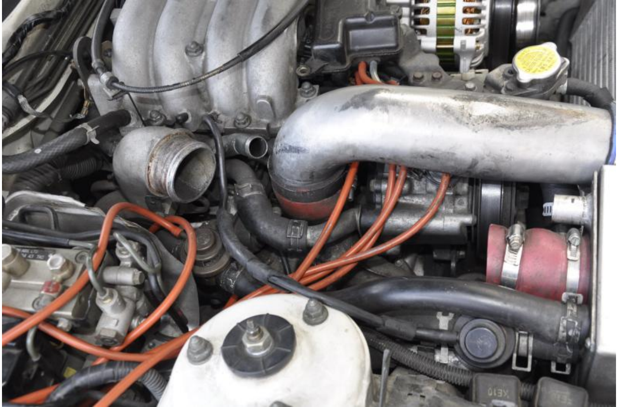
The intake pipes were removed and all hoses exposed.
