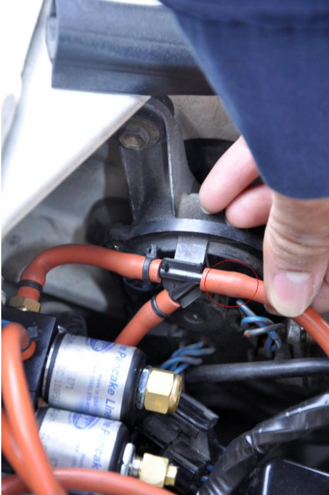
Refer to RED routing on vacuum diagram, connect from Y split and...
