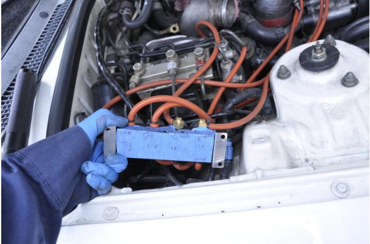
Here is another angle that showed how the solenoid rack system would be located.
