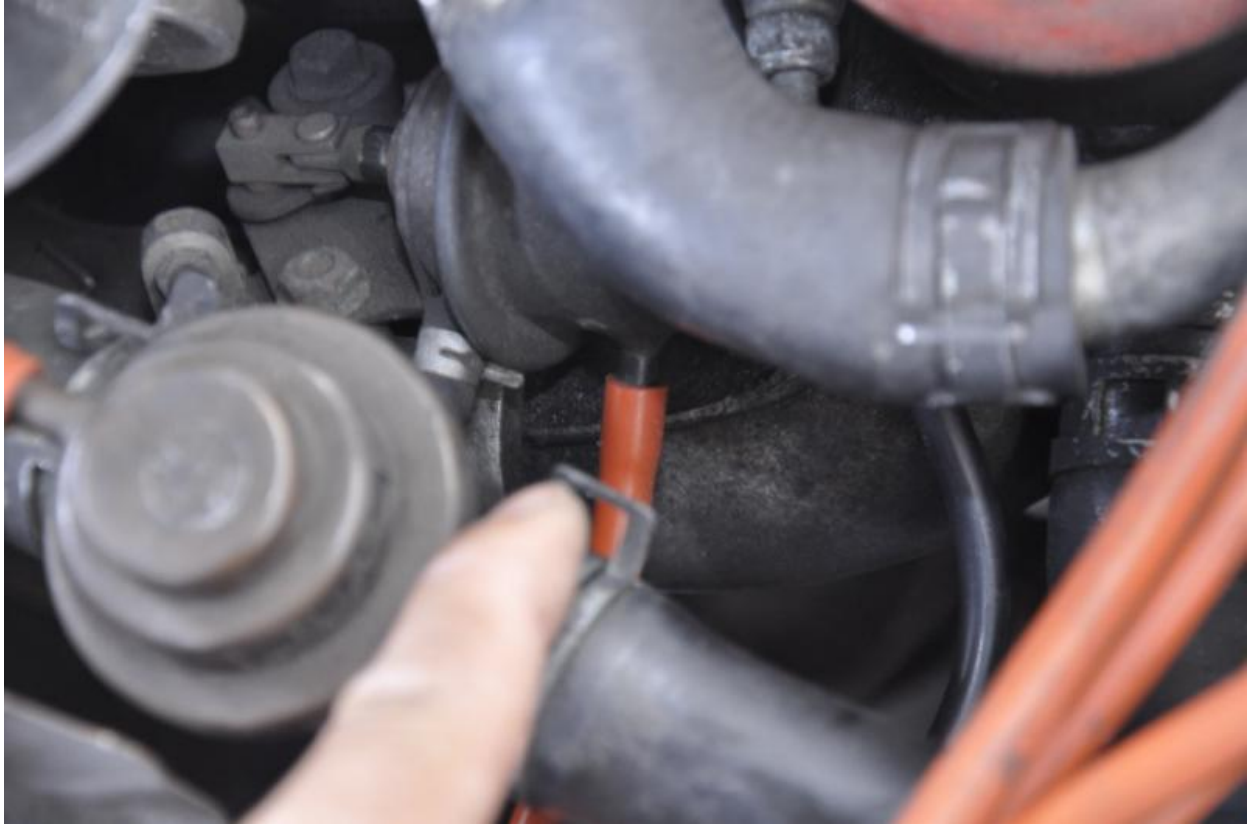
... this Wastegate Control Actuator under the intake air tube.
