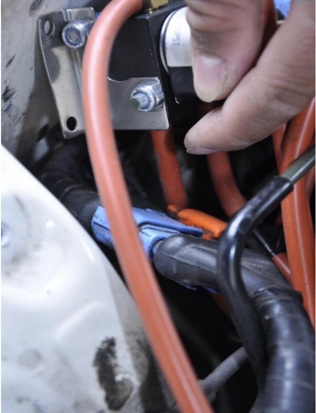
Refer to ORANGE routing on vacuum diagram, connect from port A of solenoid E to...
