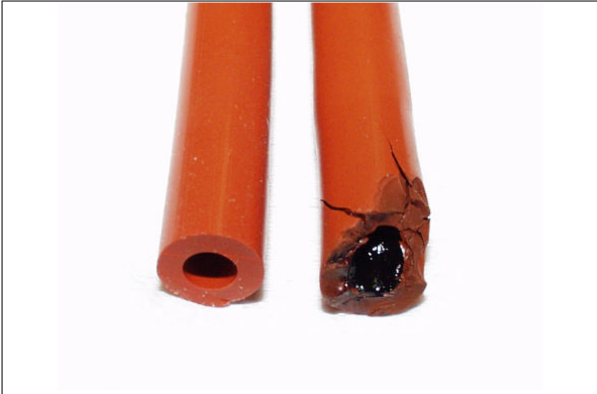
Figure 4. The silicone tubing on the left was not subjected to the hot oil. The tubing on the right was subjected to 240 °F for 1,000 hours. The tubing on the right has lost its structural integrity. It has swollen and split. It will break into small chunks if you try to pinch the tube end. The black substance inside the tube appears to be congealed oil possibly from a reaction of the oil with the silicone elastomer. This jelly like substance was not present inside the Viton or Neoprene tubing.
