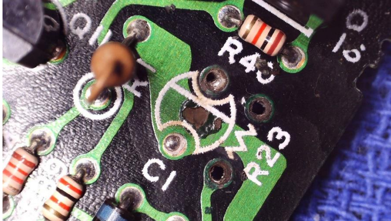
Figure 8 Damaged C1 and R23 Traces
