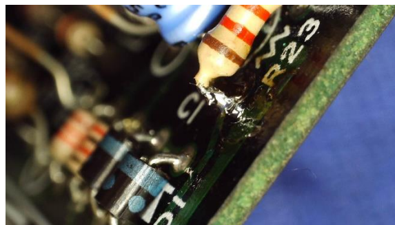
Figure 9 Large Solder Fillet for R23
