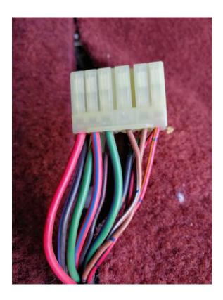
BUT, on my base S model, the subloom for the power window switch was missing, the connector attached to this loom lacked pins for the 5 wires on the left side. Perhaps this allowed Mazda to save a few dollars?
