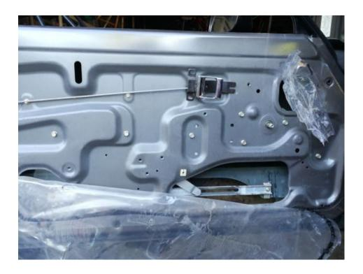
Peel back vapor barrier, a nice cool morning will make it easier to detach the adhesive putty.
