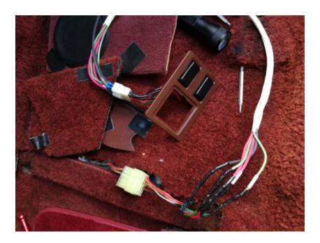
So I removed the wires from the nylon connector body and ran 6 wires of appropriate gauge to the power window switch (which is still available new from Mazdatrix!) and then ran these wires under the carpet.
