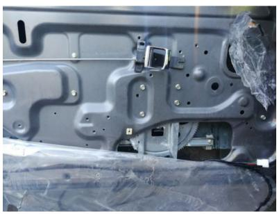
You will need more hex nuts to install powered regulators than removed with manual regulators.
