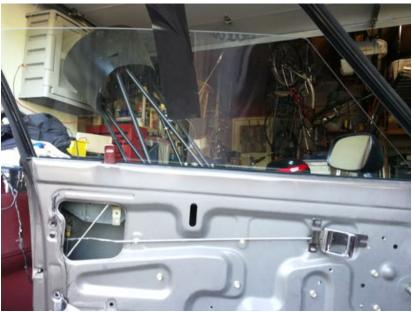
Separate glass from regulators and tape in up position to keep it out of the way.
