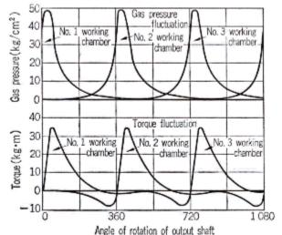
This illustration (From "The Rotary Engine", by Kenichi Yamamoto) shows gas pressure and torque fluctuation
