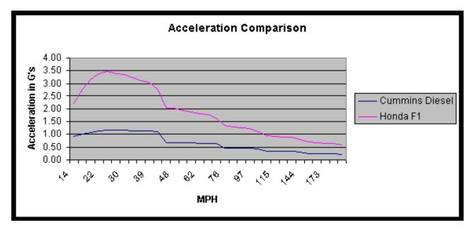
Note that at any point on the chart, the percent difference in the rate of acceleration is EXACTLY the difference in horsepower. For instance, at 200 mph, the Honda F1 engine is accelerating at a rate of .572 G's, while the Cummins diesel is accelerating at a rate of .228 G's. If we divide .228 into .572 we get 2.5, and so the acceleration rate of the Honda is 2.5 times greater than that of the Cummins.
