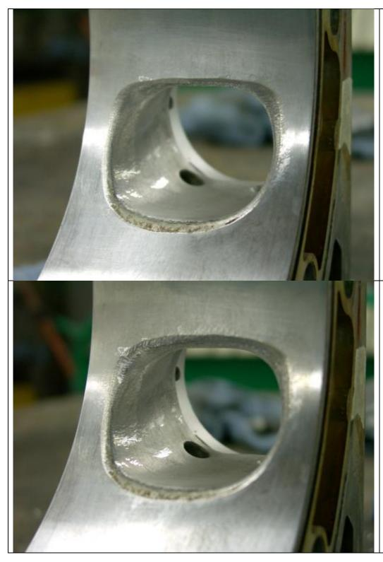
Knowing that having too large a radius on the roof of the port would hurt flow, Nathan removed some material from the flat portion of the roof, and guess what...We lost flow again!!!
