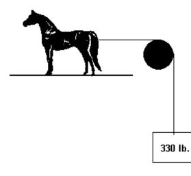
So if one horsepower is equal to 33,000 lbs.-ft. per minute, we can rearrange that to say that horsepower equals torque times rpm, divided by 5252. How do we get there?
