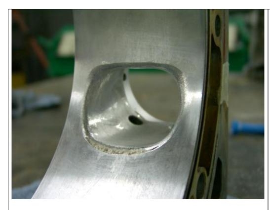
This shows the port after further squaring and widening of the roof. (If a little is good, a lot must be better!) The widening was done only at the port window, and the flow dropped to 238.3 CFM which is a 4.7% decrease.
