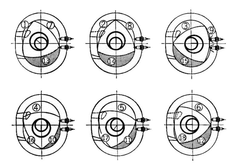
1. 45° after TDC. The chamber is slowly expanding, and the air/fuel mixture is just starting to enter the chamber. This is the beginning of the intake cycle for a conventional side port engine, and the intake port has been open for approximately 20°.
