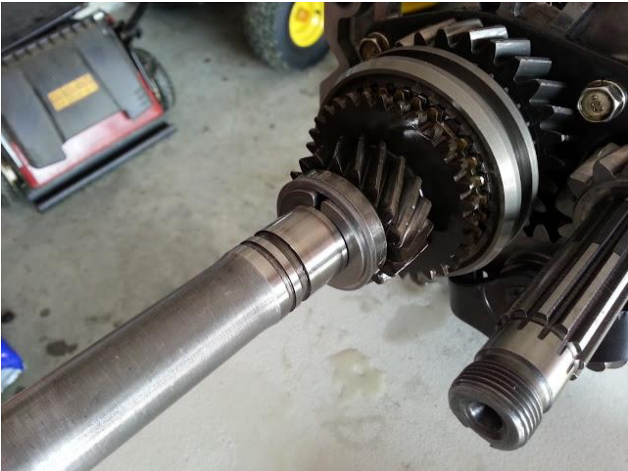
The countershaft gear slips off easily revealing a long tube spacer.
