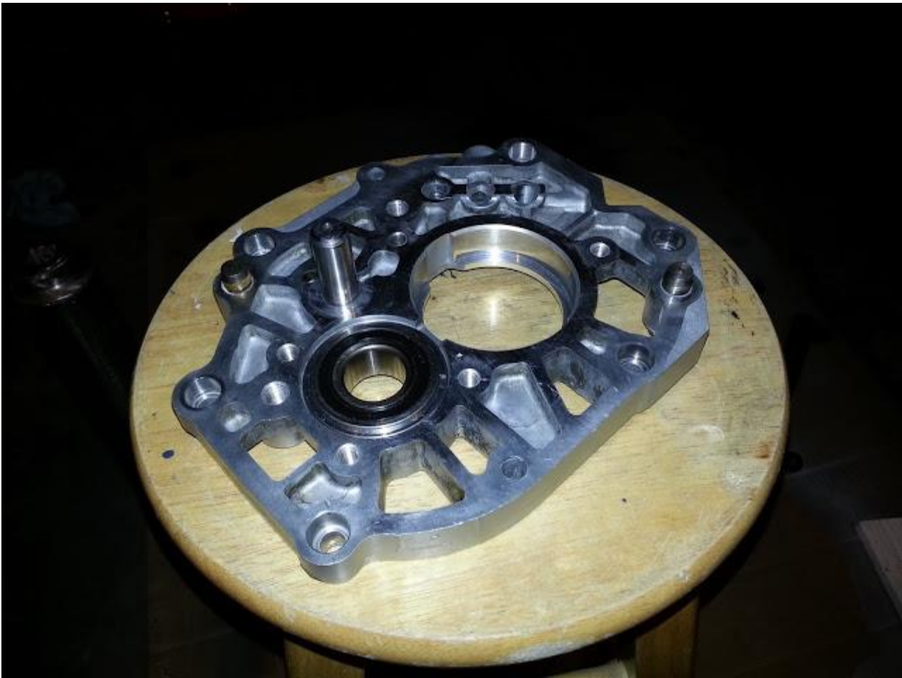
The center countershaft bearing has a c-clip around it. The c-clip does not need to be removed to push out the bearing. Both bearings removed:
