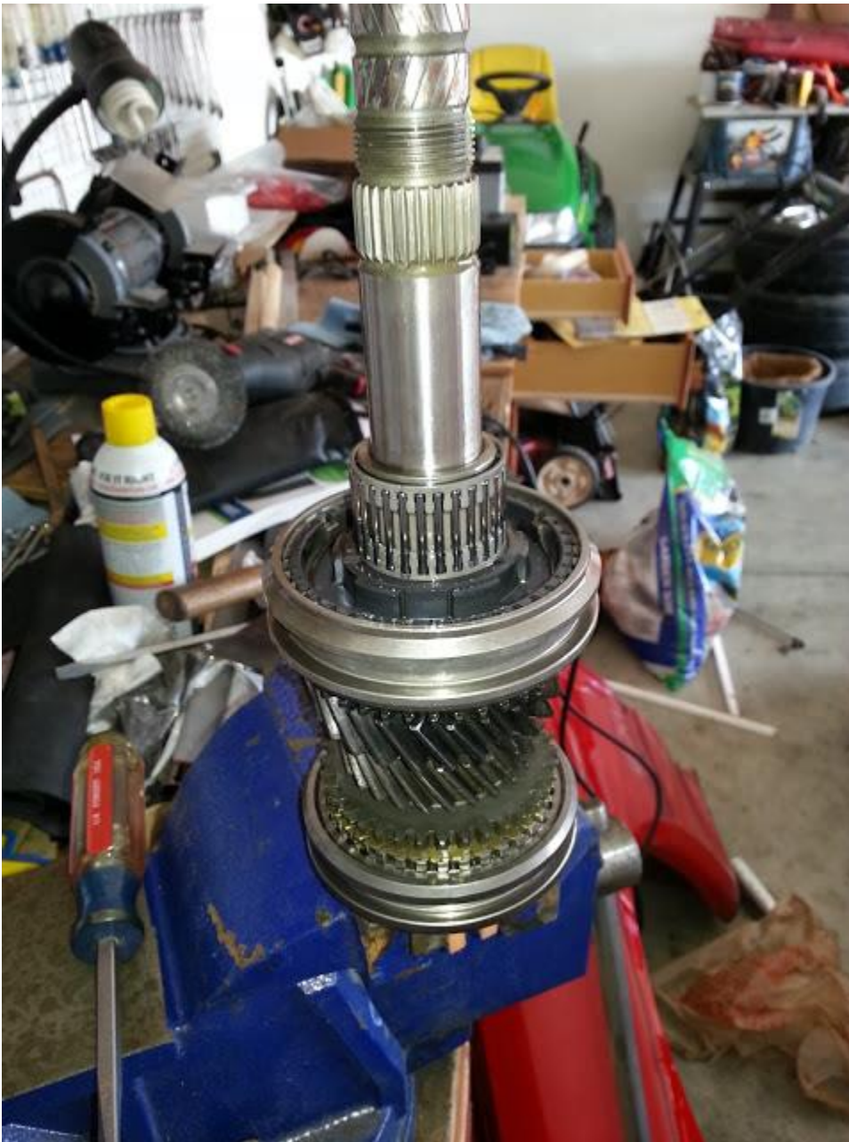
Needle bearing removed exposing inner race:
