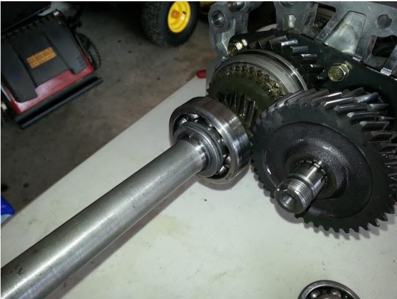
Next is the mainshaft rear bearing. First remove the c-clip.
