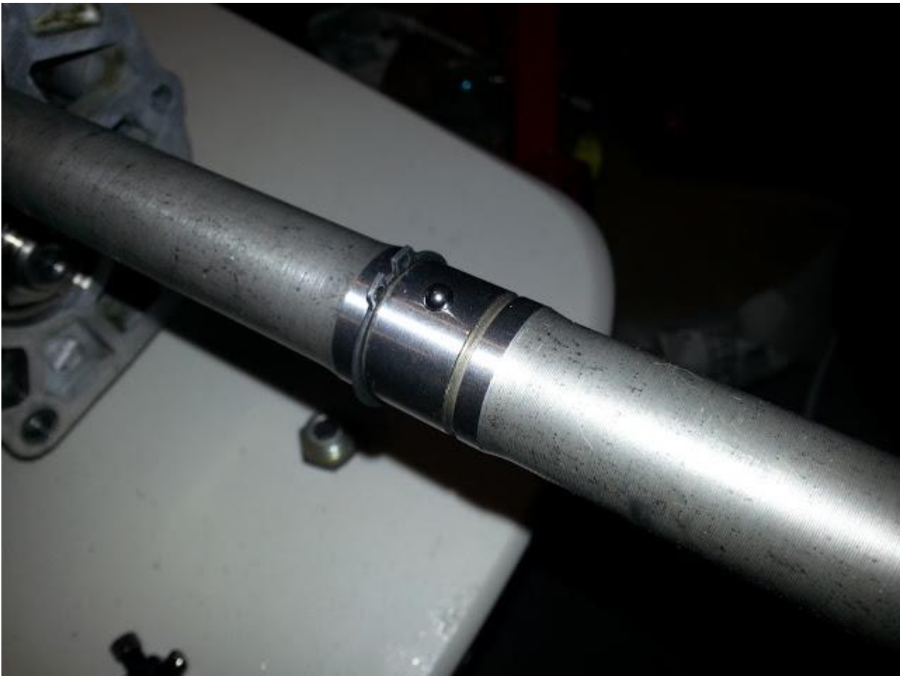
Speedometer drive gear, snap rings, and steel ball:
