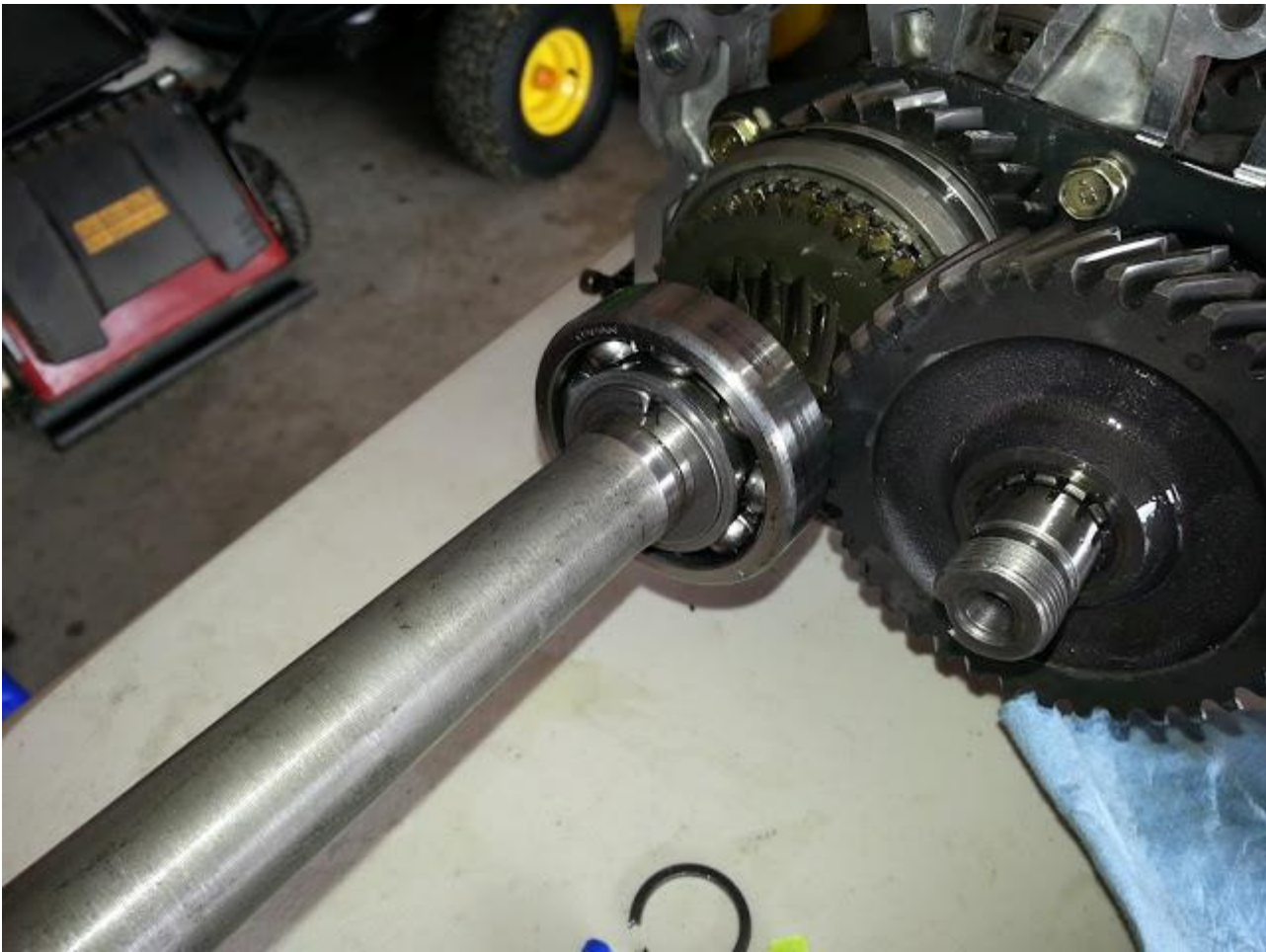
This exposes two thick c-shaped washers held by a retaining ring. Remove these to get to the mainshaft rear bearing.
