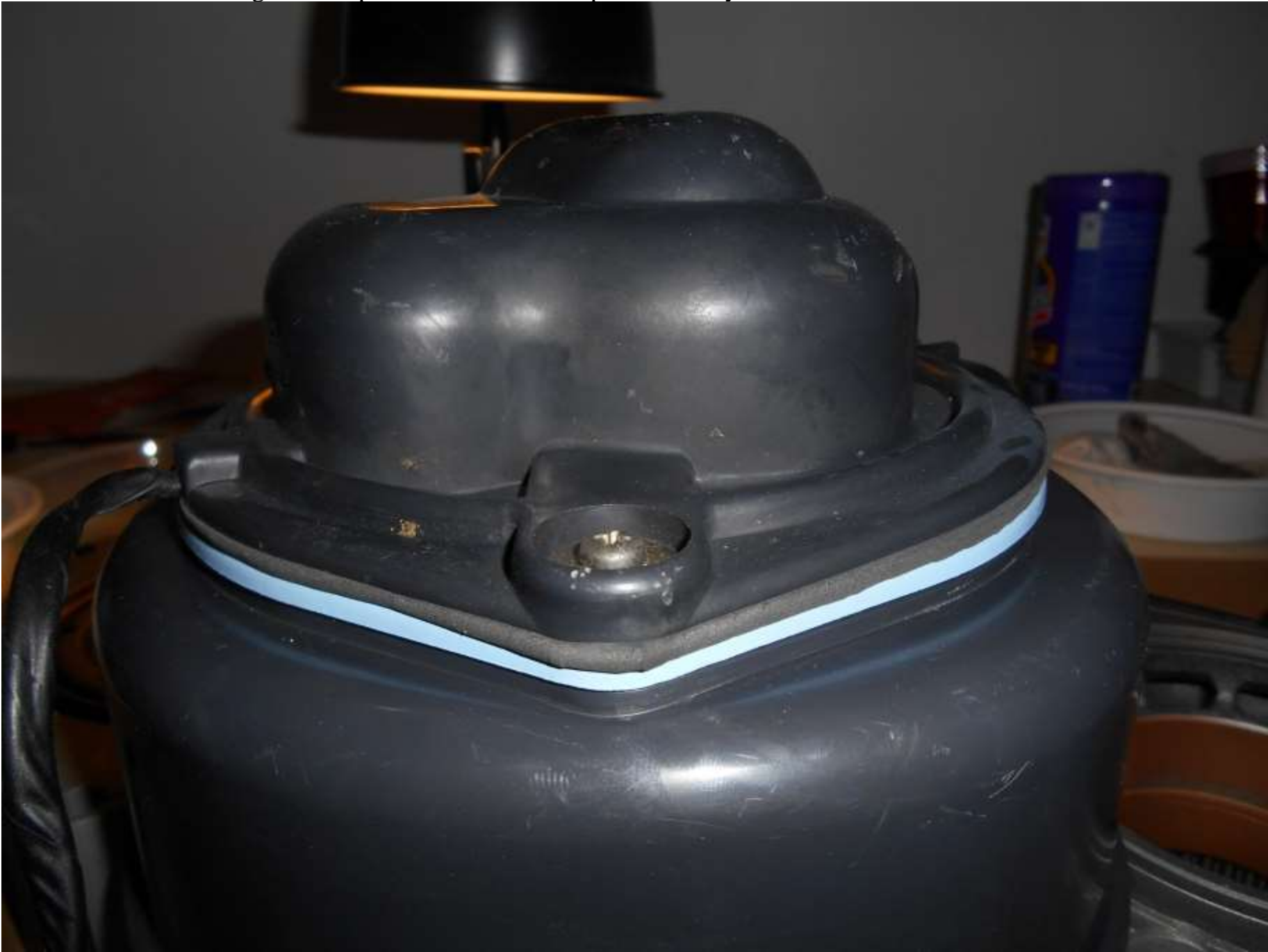
Bottom out the screws against the plastic. The foam compressed nicely.
